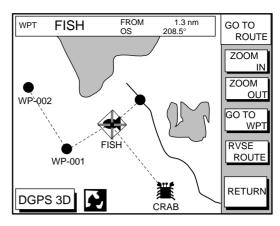
Figure 7-6 Plotter display, route selected as destination
